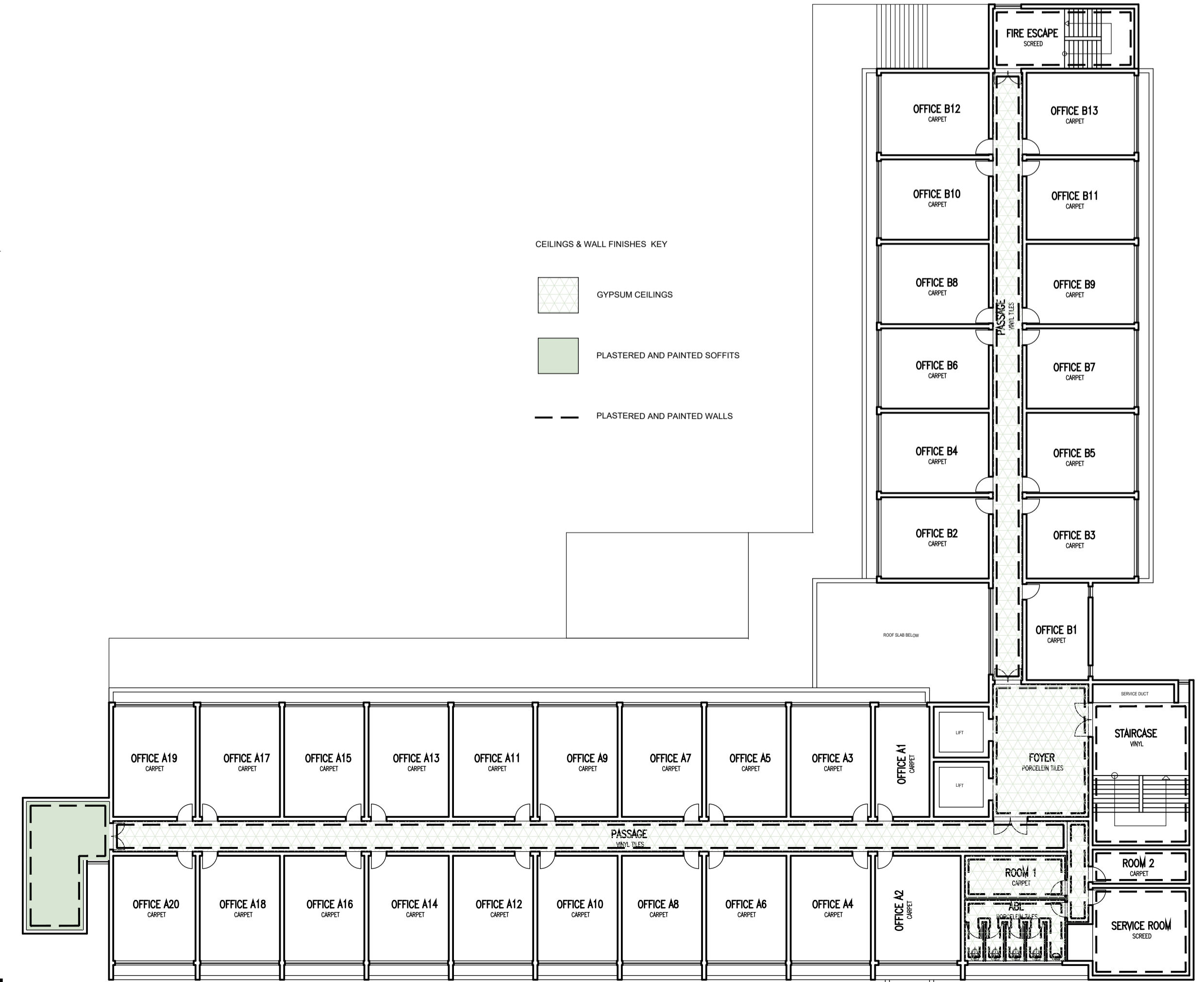
FLOOR FINISH PLANS (1st to 5th FI)- scale 1:200
