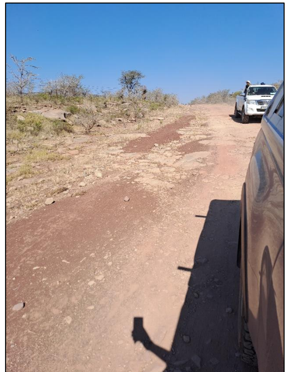
Plate 3 (Left): Deeper transported finer grained soils at TP1 and TP2. Plate 4 (Right): Sporadic rock at surface between TP5 and TP6. Note TP6 with weathered mudstone from surface throughout cut extent.
