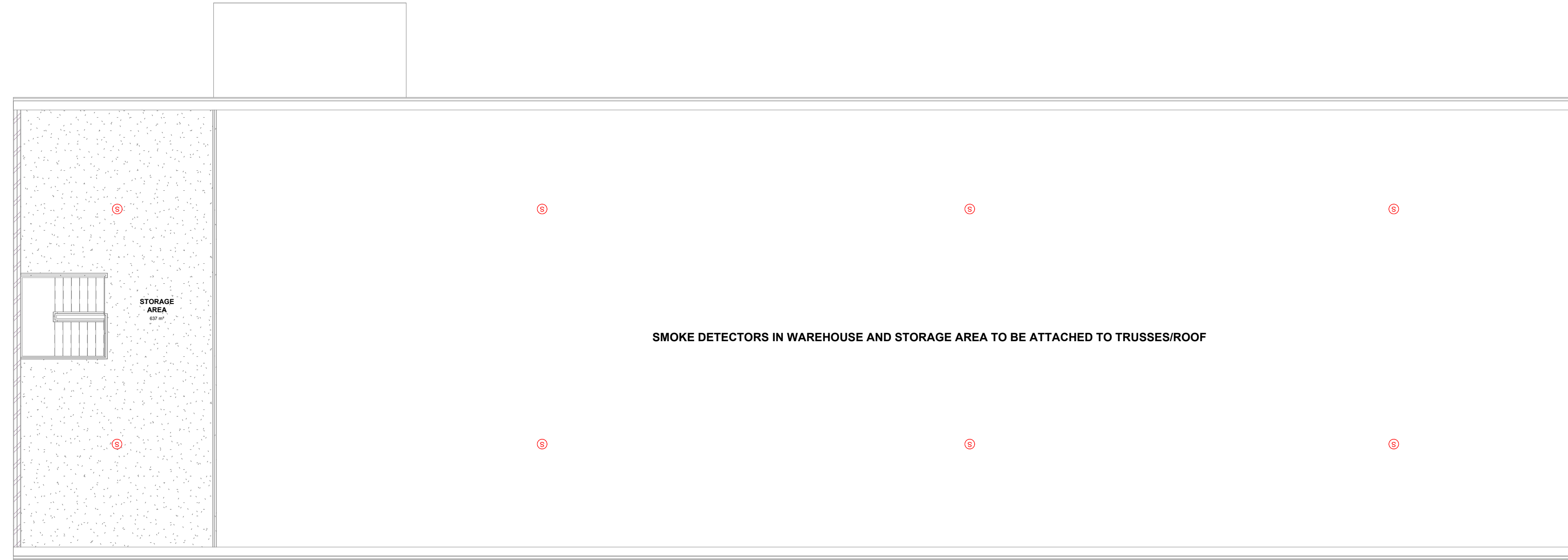
First Floor Fire Detection SCALE 1:100
